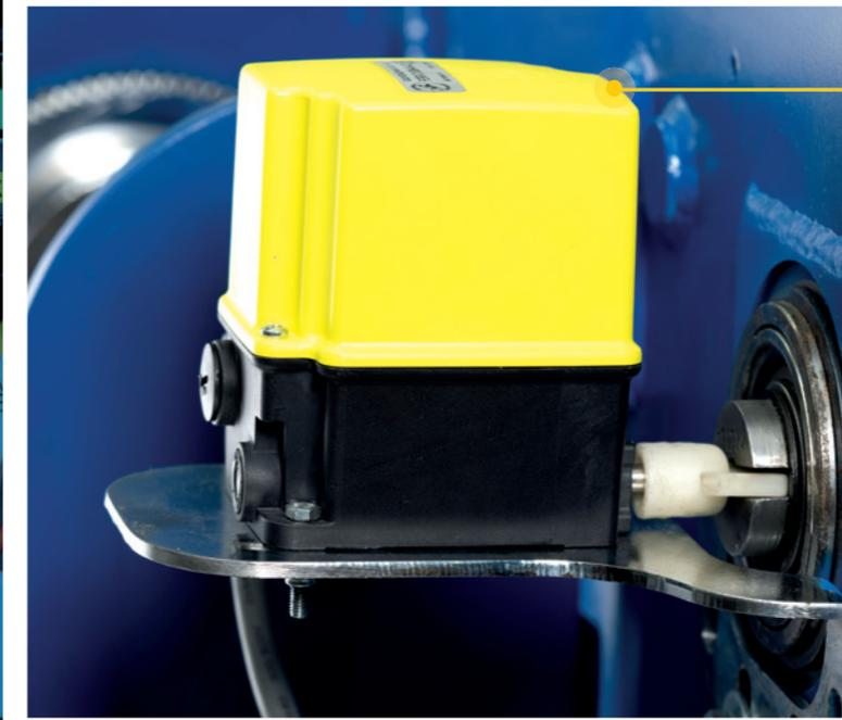
It comes equipped as standard with a compact, 4-stage stroke limit switch.
