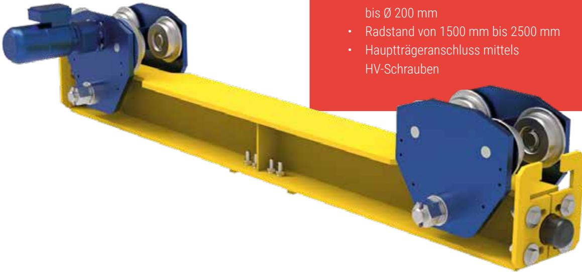
The **GCC Model GUE endtruck** is our endtruck for under running cranes. The sturdy, fully welded frame, completely machined in one set-up, is very accurate and complies with the strictest quality standards. The surface-hardened wheels are machined from solid and run extremely smoothly because of the roller bearings. This endtruck allows the use of commercially available rolled section girders, even under large loads, because the eight wheels better distribute the load.
