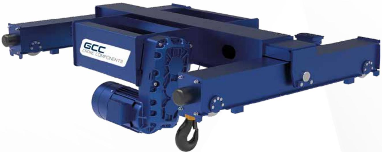
The **GCC Model DL double girder hoist** is a compact wire rope hoist for the medium capacity range. Due to the lowered design of the height, this model is the optimal solution for low room heights and lack of space above the crane main girder. A one-sided articulated running gear carrier connection ensures that all trolley wheels make full contact. In this way, the forces resulting from crane use are optimally distributed to the substructure.
