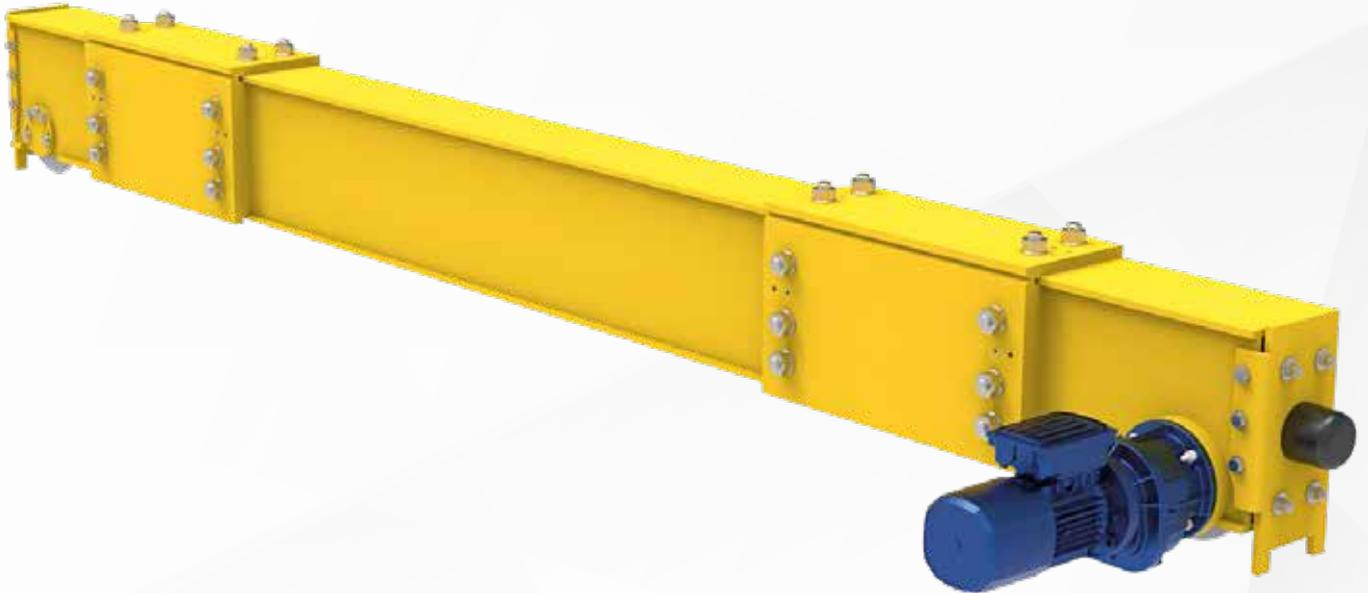
The **GCC Model GDE endtruck for double girder overhead cranes** is our endtruck for double girder overhead cranes. The sturdy, fully welded frame, completely machined in one set-up, complies with the strictest quality standards. The surface-hardened wheels are turned from solid and run extremely smoothly because of the roller bearings and the precision manufacturing.
