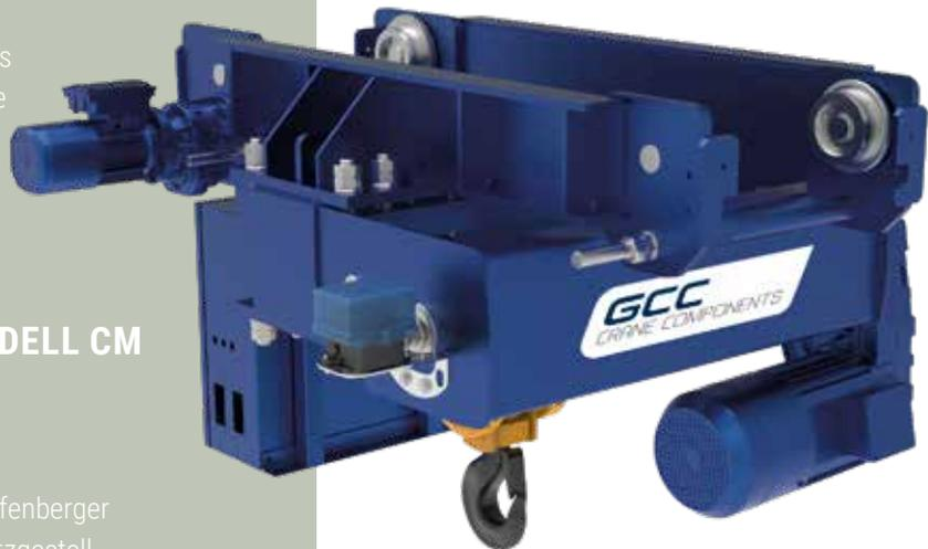
Because the rope drum is rotated through 90°, the **GCC Model CM single girder hoist** is the wire rope hoist of choice where the approach dimensions are overriding. The GCC Model CM single girder hoist is only available with rope reeving codes of 4/2 or 8/2 because of its special construction. This ensures that the load is always carried centrally.
