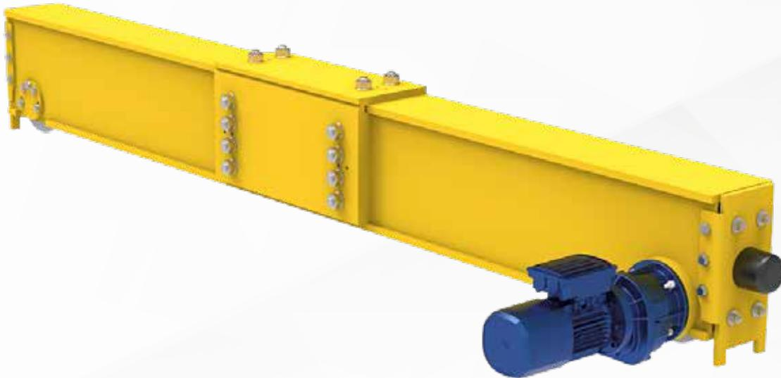
The **GCC Model GSE endtruck** is the right endtruck for single girder overhead cranes. The sturdy, fully welded frame, completely machined in one set-up, is very accurate and complies with the strictest quality standards. The surface-hardened wheels are turned from solid and run extremely smoothly because of the roller bearings and the precision manufacturing.
