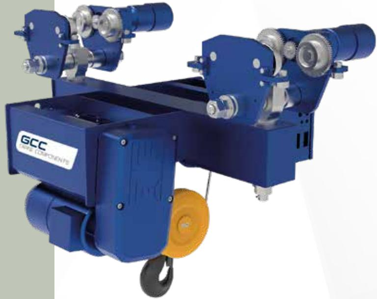
The **GCC Model SU under running hoist** is the first choice for curved single girder tracks and curve-encompassing applications. Thanks to its eight wheels, which are hinged at two points, the trolley enables the use of standard commercial rolled section girders, even under large loads. A compact, fully welded frame and the standard parallel configuration of the hoist motor and rope drum provide the low headroom that distinguish this wire rope hoist.
