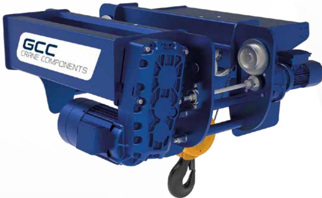
The **GCC Model E single girder hoist** is notable for its highly favourable approach and hook dimensions. These are achieved with a compact, fully welded frame adapted to provide the best match for all the components used. The parallel configuration of the rope drum and the hoist motor also contribute to the overall compact size of the Model E short trolley. In addition, this configuration ensures easy servicing and maintenance.
