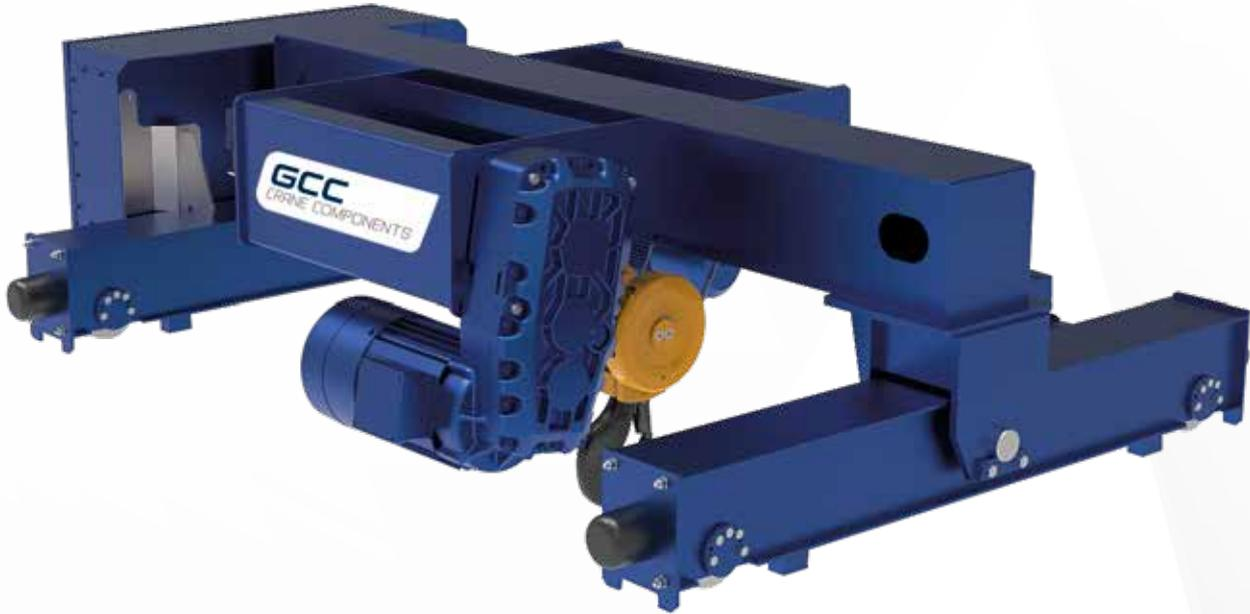
The **GCC Model D double girder hoist** is a compact wire rope hoist for the medium capacity range. The parallel configuration of the rope drum and the hoist motor makes the trolley very easy to maintain. A one-sided articulated running gear carrier connection ensures that all trolley wheels make full contact. In this way, the forces resulting from crane use are optimally distributed to the substructure.
